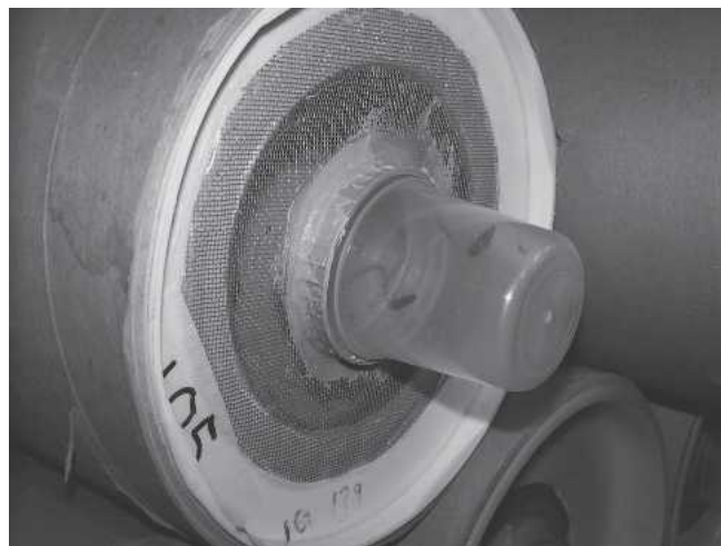
Figure 1. — Cardboard rearing tube with plastic lid, screening, and collection cup with EAB adults visible.
